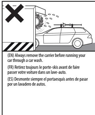
(EN) Always remove the carrier before running your car through a car wash.
