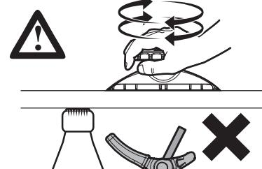
(EN) Check clamp opening for crossbar clearance. Loosen clamp thumb wheel if necessary.
